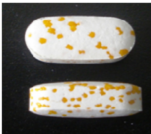
Fig. 2. Appearance of multiparticulate tablets containing 30% starch pellets and 64.5% MCC/lactose granules. Riboflavin (2%) was added as a marker to the starch-based pellets, resulting in yellow-colored pellets. (For interpretation of the references to color in this figure legend, the reader is referred to the web version of the article.)
